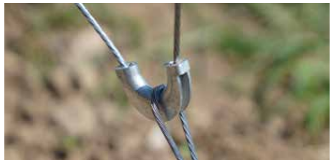
Top. Wire protector Bottom. Thimble
