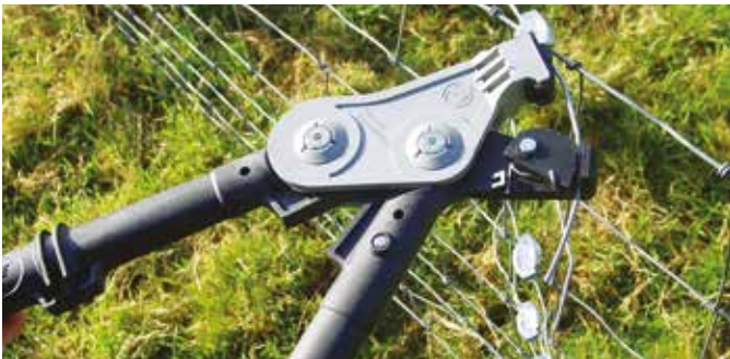
Top. Trellising with a Torq Tool 8 Bottom. Wire repair using with a Gripple Plus Medium and a Torq Tool 5
