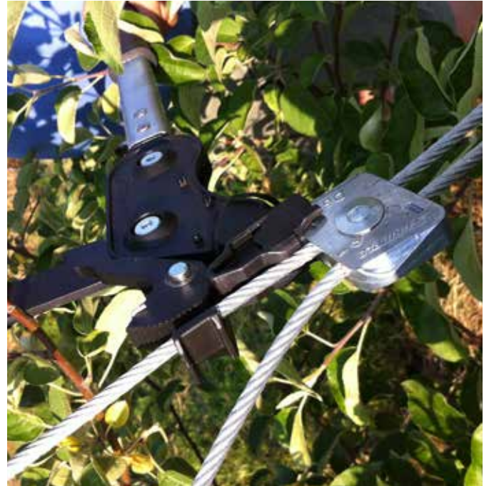
Dynamic 6 - Tensioning using Contractor Tool.
