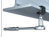
Tighten the bolt using a torque wrench or impact driver until the head shears off. Bolt will shear-off when torqued to 29.5 lb-ft (40Nm). The bolt tip will be securely embedded into the beam.
