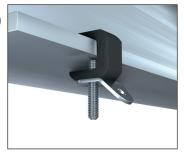
Position the bracing bracket on the underside of the clamp in the plane desired, slide washer and then tighten the nut to secure bracket in place.
