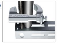
Hold and press the conduit clip to open the jaw. - fit around the rod then conduit.
