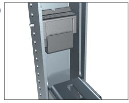
To install the bracket, support the bracket's weight and press the cartridge's button to retract the fixing pins. Hold the cartridge button whilst locating the bracket into the pendant's channel. Release the cartridge button to allow the cartridge's pins to locate the pendant's holes (ensuring that the pin has passed all the way through the hole and the locked line is visible).
