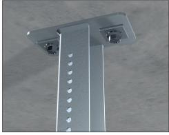
To install the pendant, mark out the hole centre locations, using the top plate dimensions (page 2). Drill the fixing holes to the required depth and diameter\*. Position the single pendant over the drilled holes and anchor into place, if necessary use a square washer underneath the fixing.
