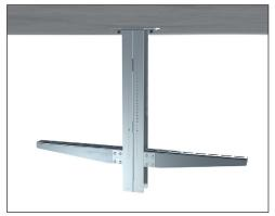
Repeat steps 1-3 above for the installation of Backto-Back pendants. When installing multiple brackets at different heights, ensure a 187.5mm gap is left between horizontal supports.
