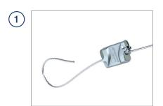
Insert the wire rope through insertion channel
