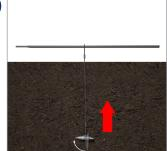
When PV Anchor is at desired depth, use JackJaw to remove drive rod (can also be done by hand in softer ground) before using JackJaw and Anchor set tool to load lock PV Anchor.
