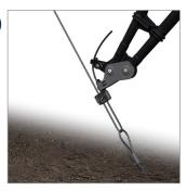
Using the Gripple Torq Tool, apply 100kgf via the tail wire.
