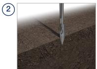
Push the PV Anchor in to the surface of the ground at prescribed location.
