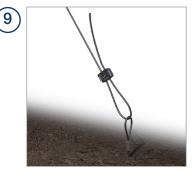
Feed the fused wire through the anchor thimble and back through the dynamic tensioner. Pull hand tight leaving min. 150mm tail wire to remove as much slack as possible.
