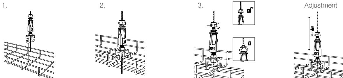
Maximum off axis suspension = 15° (Unless otherwise specified by Gripple Technical Services).
