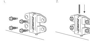
Use No. 8 self drilling screws (not supplied). Ensure a minimum 3" / 75 mm of cable exits the hanger.
