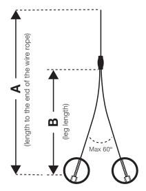
Dimensions A and B should be specified along with the required end fixing.
